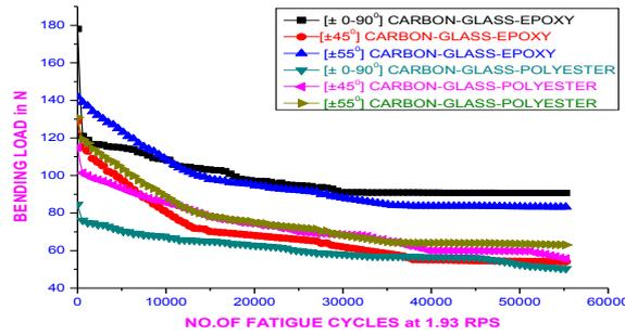
\*RESIDUAL STIFFNESS VALUES OF  $[0^0.90^0]$ ,  $[\pm 45^0]$ , AND  $[\pm 55^0]$  ANGLE PLY ORIENTATION SEQUENCE OF STACKING OF CARBON-GLASS-EPOXY & CARBON-GLASS-POLYESTER
