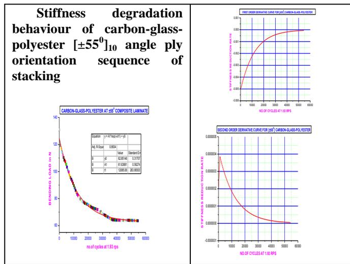
CONSOLIDATED FLEXURAL FATIGUE TEST RESULTS OF  $[0^0.90^0]$ ,  $[\pm 45^0]$ , AND  $[\pm 55^0]$  ANGLE PLY ORIENTATION SEQUENCE OF CARBON-GLASS-POLEYSTER HYBRID  $[\pm 0-90^0]$
